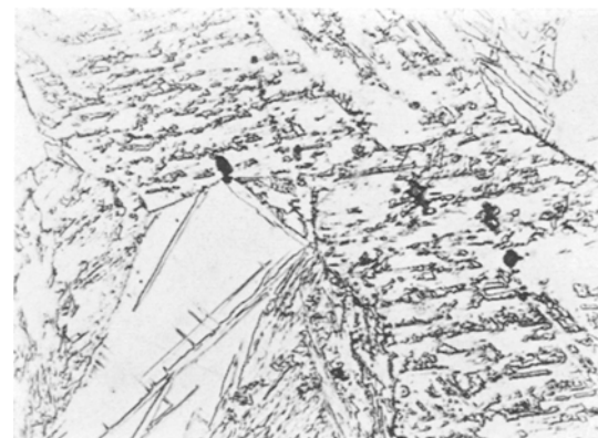
Figure 8 Steel S4, 1200°C – 15 min ( \times 350 ).
